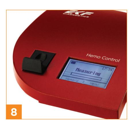
The measurement will begin when the cuvette holder is closed.
