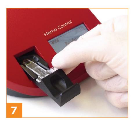
Open the cuvette holder by pulling it out carefully. Insert the cuvette with the raised wing pointing to the right of the cuvette holder.
